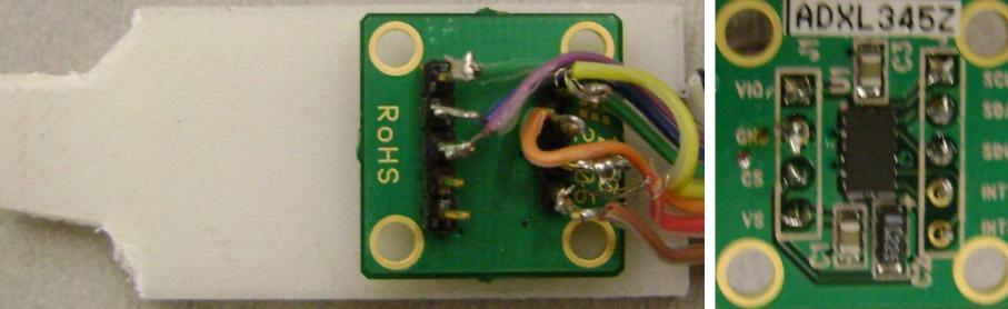
Left: the plastic fingernail with the attached accelerometer. Right: the other side of the accelerometer board (the ADXL345 is in the center).
